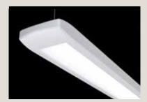
The Peerless Proper by **Acuity Lighting** is a suspended linear direct/indirect luminaire with a 5-in. wide aperture allowing outputs up to 1,200 lumens per ft direct, and 1,500 lumens per ft indirect, the highest output in a combination luminaire. It is available in single or two-circuit configurations with an efficacy ranging from 105 to 143 lumens per watt.
