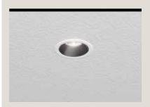
Zaniboni Lighting introduces the Mini RD Downlight, the smallest beveled aperture that utilizes a unique drywall anchor installation method. It has a 1.1-in. aperture diameter with a beveled trim. The top part of the trim screws into drywall, and the light engine plugs into the driver and pushes into the trim.
