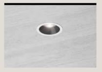
Also from **Zaniboni Lighting**, the Mini RX Downlight is the smallest beveled aperture that utilizes a unique screw-in bolt action installation method for wood or stone ceilings. The Mini RX has a 1.1-in. aperture diameter with a beveled trim. The top part of the trim screws into a retaining nut above the wood or stone ceiling and the light engine plugs into the driver and pushes into the trim.
