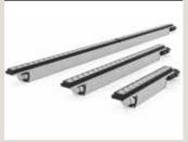
The CoviO Graze from **Cooper Lighting Solutions** provides the highest light output for an outdoor accent luminaire of over 1,500 lumens per foot and an industry leading 112 lumens per watt. It provides wall washing and grazing lighting with more than 9 optical distributions and an integral driver. The fixture has 94 CRI, and is available in four correlated color temperatures. It can dim down to 1% with phase and 0-10-V controls.
