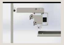
The S330 from **The Lighting Quotient** is the only recessed-pocket luminaire with fully adjustable linear optics in a choice of single or dual heads. The heads are fully adjustable and lockable, allowing smooth aiming for walls up to 40 ft tall. Specifiers may elect to include one row of static white and one row of RGBW for maximum versatility. Aperture width is field adjustable from 4 to 6 in. or 9 to 12 in.
