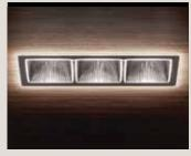
Crystal by iGuzzini North America is the first recessed luminaire to use Opti Diamond technology as a unique way to light up the ceiling and the floor. This technology that adopts the catadioptric principle, revolutionizes the visual perception of space and enhances well-being, and has an efficacy 140 lumens per watt. The frame gathers the light emitted by the reflector and spreads it over the ceiling, thereby combining décor and function for even better spatial distribution.
